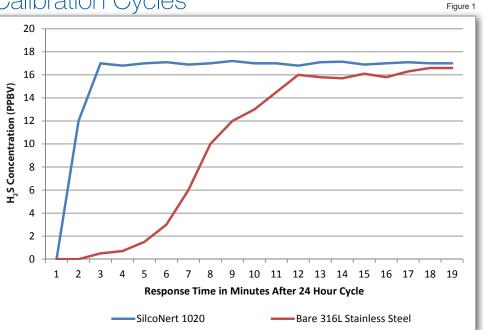
Figure 1 compares the response time of a calibration gas containing 17 ppbv of hydrogen sulfide delivered through a 316L stainless steel regulator and a CONCOA SilcoNert 1020 regulator after 24 hours. In this typical scenario, calibration was more than 10 minutes faster with SilcoNert 1020 than with 316L stainless steel.
